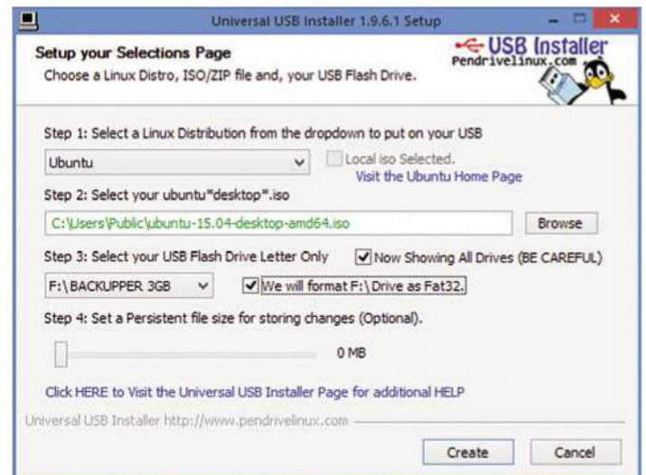
▲ No optical drive? Save Linux to a USB flash drive and boot it from that
